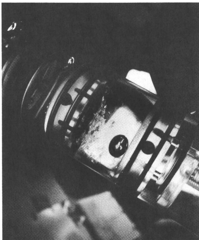
Figure 2. Photograph of Lead Iodide Crystals Grown Aboard the Discovery Shuttle Mission
