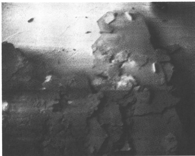
Figure 6. Auger Image of Shuttle Grown Lead Iodide Crystals
